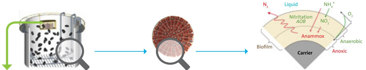
The presence of retention grids with a suitable meshing avoids any loss of carriers out of the reactor and **guarantees process safety over time.**
